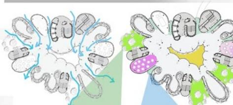
THE DIAGRAMS ABOVE SHOWS HOW MIND IS FLOWING INTO EACH FLOORS THROUGH CROSS VENTILATION. THE FLOW OF THE WIND EXCHANGED THE INSIDE AIR WITH THE OUTSIDE AIR. STALE AND DIRTY AIR WITH BACTERIA WILL BE ELIMINATED OUTSIDE.
