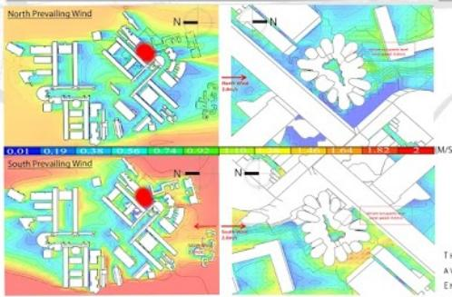
THE SITE HAS TWO PREVAILING WIND THAT BLOWS FROM NORTH AND SOUTH. SIMULATION SHOWED THE PREVAILING WIND FROM THE NORTH DIRECTION BLOW WITH THE SPEED OF 2.0 M/S AND 0.8 M/S ON THE INTERIOR OF THE HUB. ACCORDING TO THE MS 1525, THE MINIMUM LEVEL OF WIND SPEED TO ACHIEVE THE COMFORT LEVEL IS 0.6 M/S. SO, DURING THIS SEASON, THE USER WILL FEEL COMFORTABLE INSIDE THE BUILDING.
