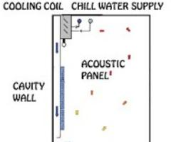
PDV RELIES ON NATURAL CONVECTION OF HEAT TRANSFER. THAT IS WHEN THE WARM AIR RISES AND BE PULLED INTO THE AIR DUCTS ON THE WALL. THE WARM AIR IS COOLED BY THE COOLING COILS THAT HAS CHILLED WATER RUNNING INSIDE IN CYCLES. THEN, THE COOLED AIR WILL FLOW DOWN THROUGH THE CAVITY WALLS AND RETURNS INTO THE ROOM. DUE TO THE LOW VELOCITY OF THE SUPPLY AIR, UNDESIRABLE DRAFT IS ELIMINATED, LEADING TO GREATER OCCUPANT COMFORT. THIS SYSTEM ALSO BRINGS A LOT OF BENEFIT SUCH AS:
