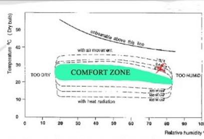
THE WARM SEASON IN SINGAPORE IS AROUND APRIL OR MAY, WHICH HAS AN AVERAGE HIGH OF 31.7°C AND LOW OF 24.4°C ACCORDING TO THE NATURAL ENVIRONMENT AGENCY (NEA). WHEREAS THE WIND VELOCITY INSIDE THE BUILDING RANGED FROM 0.35M/S (NORTH WIND) TO 0.9M/S (SOUTH WIND). ACCORDING TO MS1525, THE COMFORT RANGE FOR AIR VELOCITY RANGE AROUND 0.5M/S<sup>1</sup> TO 1.0M/S<sup>1</sup>. WE CAN ASSUME THAT THE DRY BULB TEMPERATURE (DBT) OF THE INTERIOR OF THE NTU LEARNING HUB HAS REACHED THE COMFORT ZONE.
