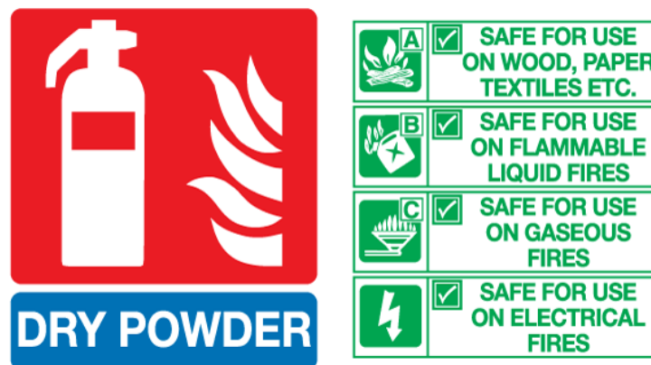
Figure 5.49: The characteristics of dry powder fire extinguisher
